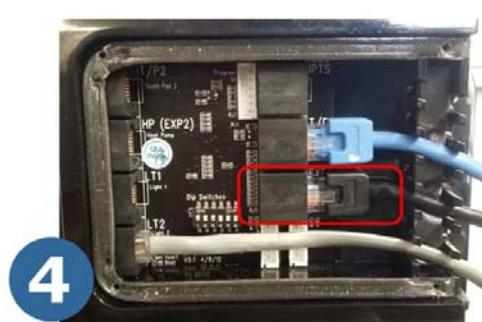
**4** Connect black data cable from SpaLINK module into EXP1 socket
